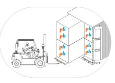
The packs stand on the metal sheets. Use lifting equipment to pull the packs of sandwich panels out of the container by the special fasteners on the metal sheets.
